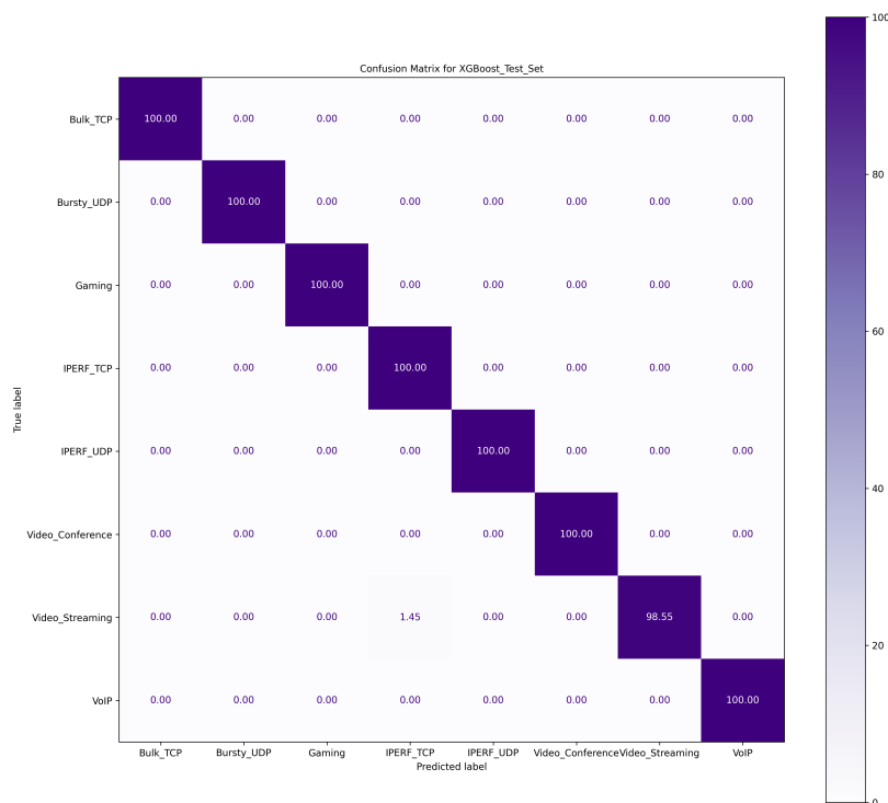
Figure 9: Confusion Matrix – Testing Ethernet Channel
