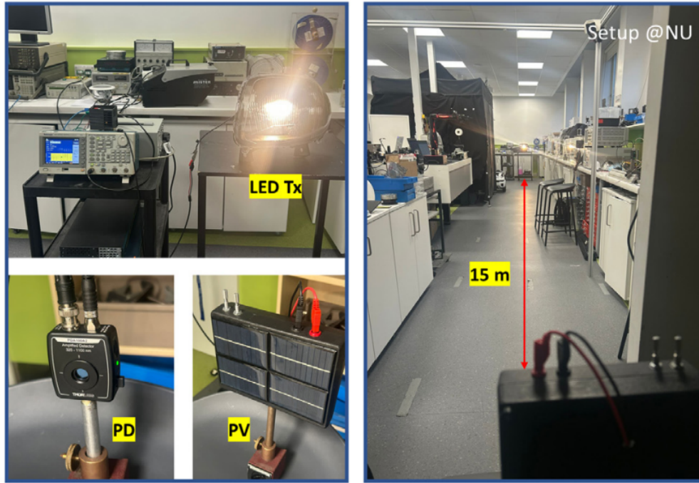
Figure 10. VLC link testbed at NU, LED transmitter with signal generator and PD/PV-based Rx's at 15 m line-of-sight for a proof of concept vehicular to infrastructure communications.
